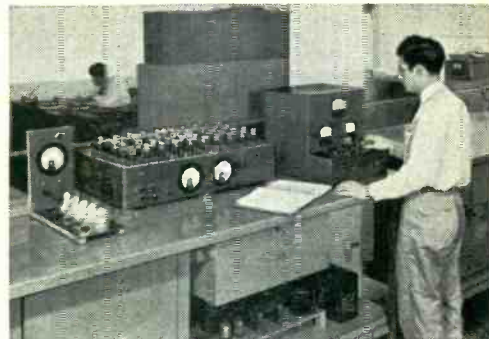
Electronic Engineering — Life test rack and emission test set. Checking Superior assembled standard diodes under simulated customer conditions to determine if material meets minimum requirements.
