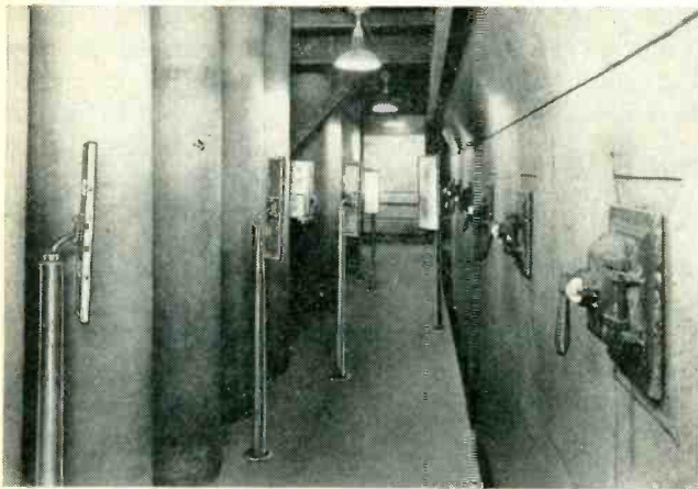
Arrangement of mirrors and camera pickup at left enables operator to look into six furnaces at a glance on remote monitor screen at extreme right
