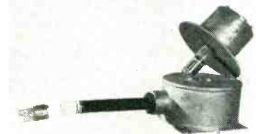
Light-piping device for remote detection of radioactivity using an anthracene crystal coupled to a 1P21 multiplier phototube by a lucite rod
